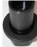
threaded area of the nut. Remove any nut from service where the scribe line enters past the threads (not flange washer) and contact the manufacturer for dimensional specifications.
