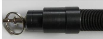
over the threaded end of the stud. If the stud enters the gauge more than the first 4-5 threads, replace it and contact the stud manufacturer for specifications.
