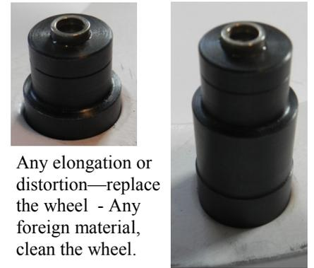
Any elongation or distortion—replace the wheel - Any foreign material, clean the wheel.
